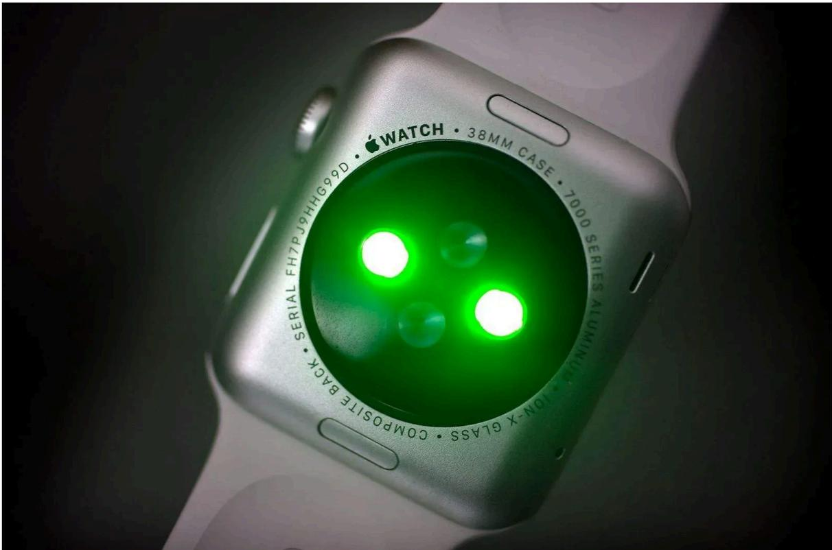
In recent years, we have seen lots of new wearable devices getting equipped with ever more advancing sensors. One of the most commonly used sensors is PPG(Photoplethysmogram). This sensor is capable of Monitoring heart rate and cardiac cycle respiration, blood pressure, and SpO2(saturation of partial pressure oxygen)providing an insightful tool to assess our health. Its small size and versatility makes it invaluable to everyday healthcare. So how does it work?
